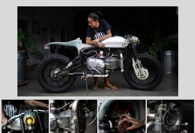
**FRAME & SUSPENSION**: Both swing arms are stretched and fitted with single-sided suspension from a gas tension spring and an opposing enclosed coil spring. The subframes on these bikes are mirrored to each other. The white bike's frame loops around to the front, and the black bike's frame continues to the rear. The main frame on both bikes had the secondary down tube removed and then was reinforced with gussets.
